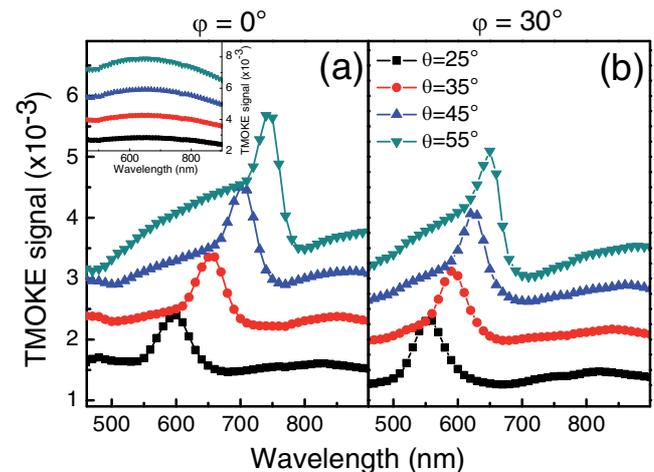
**Figure 2** (online colour at: [www.pss-rapid.com](http://www.pss-rapid.com)) TMOKE signal as a function of the wavelength and incidence angle  $\theta$  for the two crystal orientations. The inset in (a) is the TMOKE corresponding to the continuous Fe film.
