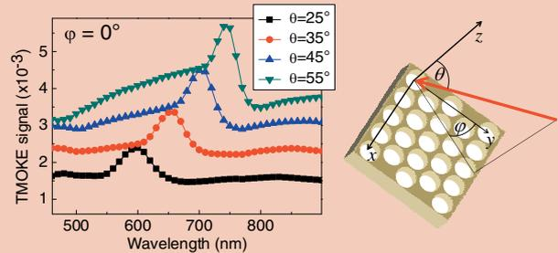
Schematic representation of the system, and TMOKE signal for a Fe membrane along  $\varphi = 0^\circ$ .
