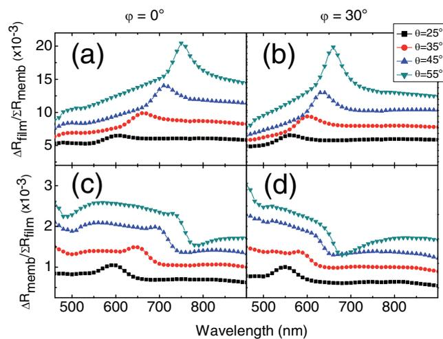
**Figure 3** (online colour at: [www.pss-rapid.com](http://www.pss-rapid.com)) Modified TMOKE signal for different incidence (polar) angles along the two high symmetry lines  $\varphi = 0^\circ$  and  $\varphi = 30^\circ$ , respectively.
